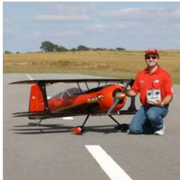
The spec.'s call for a DA-100 engine and show the aircraft weighing about 26 lbs. with an 89" wingspan.
