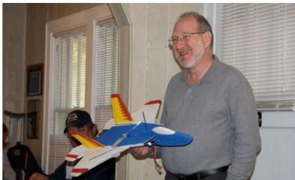
KC Moore was in attendance and was carrying several new aircraft. Here is a scratch built A-4 that he built. It features a \$10 China motor, a ¼" balsa wing, CC 25 amp ESC, and 3S 1500 mah power.
